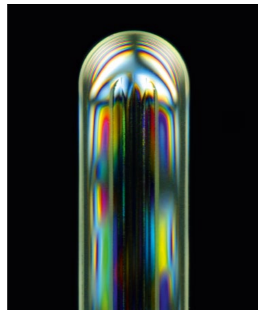
Special tempered MAXOS ® glass under polarized light
