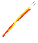
Braided fiberglass conductor insulation, glass fiber over each wire, impregnated in order to prevent raveling. Accuracy according to IEC 584 Class 1. Solid conductors 0.711mm diameter, and approximately 1.7mm outer diameter per wire, twisted together.Suitable for making thermocouples for high temperature applications in the steel and alumiumindustrie, foundries, furnace research, welding, foundries and heat treatment. Measuring range -60 °C to 650 °C with 750 °C peak.
