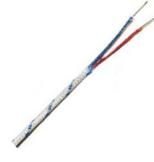
Braided Glassfibre wire insulation, laid side by side. Glassfibre braided overall, impregnated with a silicone varnish. Accuracy conforms to IEC 584. 0.2mm wires dimensions 1.2x1.9mm, 0.5mm wires dimensions 1.7x2.5mm, 1.0mm wires dimensions 2.2x3.4mm. Ideal for making thermocouples and suitable for a variety of high temperature applications in steel and aluminum industry, casting, heat treatment, component testing, furnace surveys and welding control. Option: Stainless steel braided overall.
