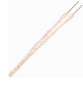
Solid type K thermocouple wires 0.8mm each. Accuracy conforms to IEC 584. Braided Ceramic fibre wire insulation. Each conductor laid side by side and braided with Ceramic fibre. Overall with Ceramic fibre braided. Overall dimensions 2.9 x 4.5mm Ideal for making thermocouples and suitable for a variety of high temperature applications in steel and aluminum industry, casting, heat treatment, component testing, furnace surveys and welding control.
